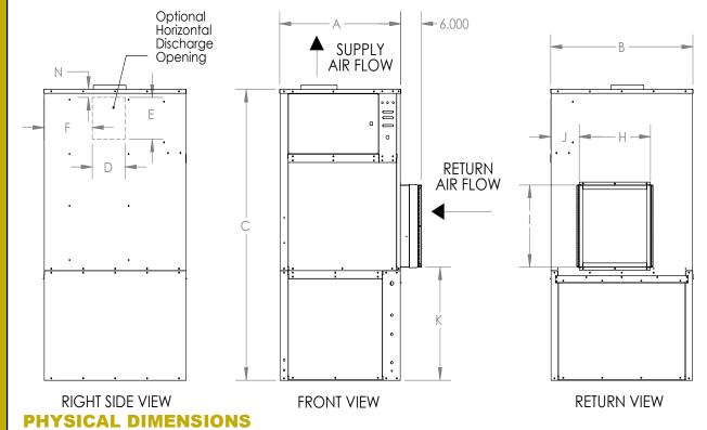
AIR COOLED - NON WATER HEATING DEHUMIDIFIERS DCA 650TV WATER HEATING ASSIST DEHUMIDIFIERS DCA 650TVWH
